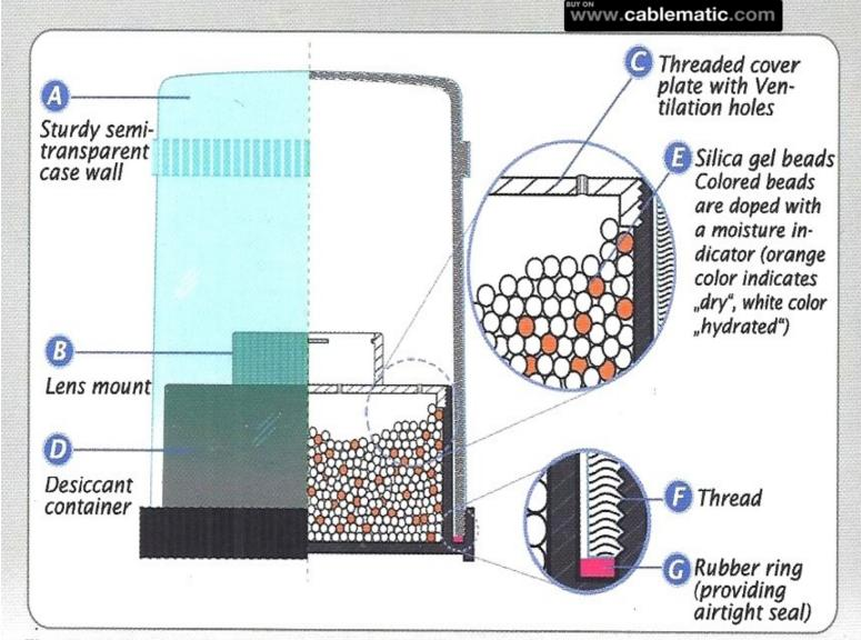
The about 2,5mm thick Case Wall (A) is made of semitransparent, high strength, antistatic plastic. It protects the camera lens against damage by all kinds of pressure, impacts, dirt, dust, water, mud or by electrostatic discharge in heavy duty outdoor employments in difficult climates.
